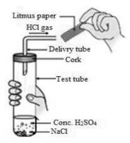
Blue litmus paper is brought near the mouth of the delivery tube to check the presence of acid but no change is observed in the color of litmus paper because:
